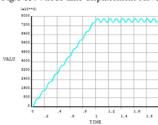
Fig.10 8574 node time- stress curve
